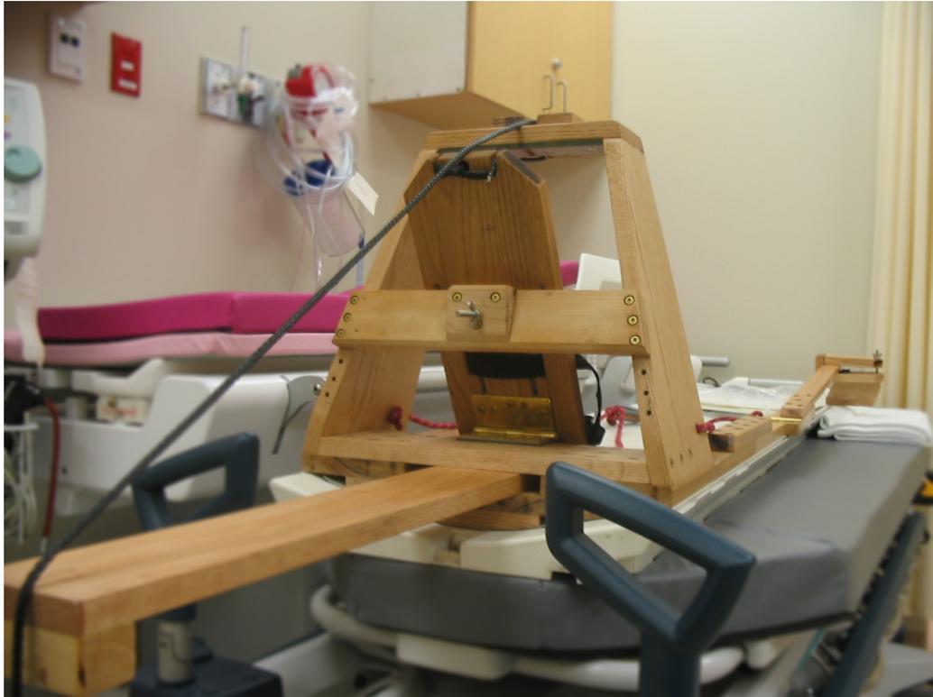
**Figure 8.27: Pulley Ergometer.** The ergometer features a pulley system connected to a weight load to vary the contraction force.
