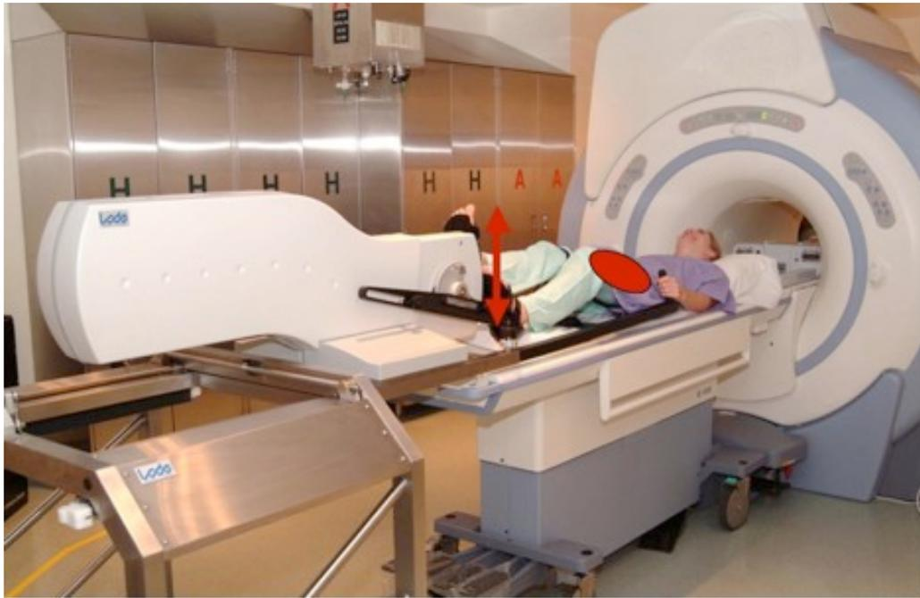
**Figure 8.28: Lode ergometer.** The MRI compatible ergometer allows dynamic power adjustment.
