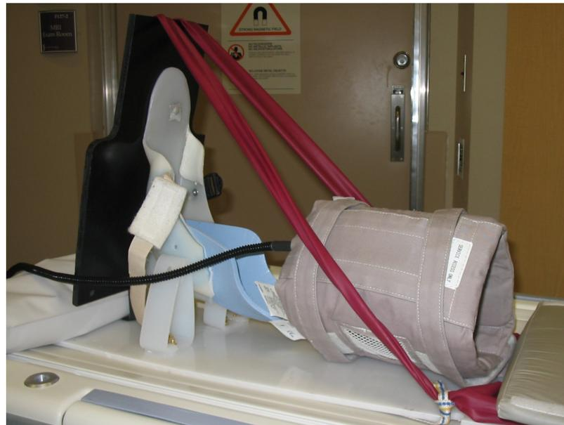
**Figure 5.13: Elastic ergometer photo.** Thera-Bands are set for resistance, and the flexible surface coil is ready to accept a subject's leg.
